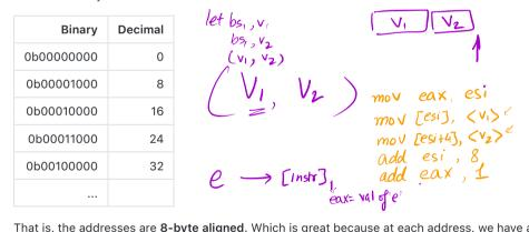
That is, the addresses are **8-byte aligned**. Which is great because at each address, we have a pair, i.e. a **2-word = 8-byte block**, so the *next* allocated address will also fall on an 8-byte boundary.
