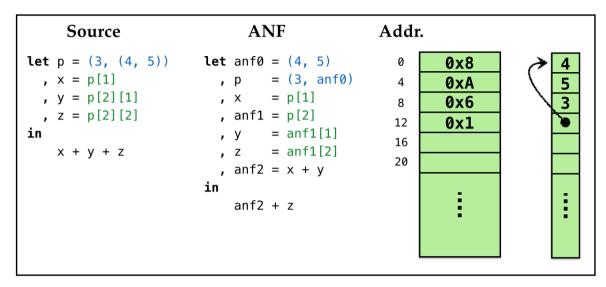
Lets work out how the values corresponding to x, y and z in the example above get stored on the stack frame in the course of evaluation.
