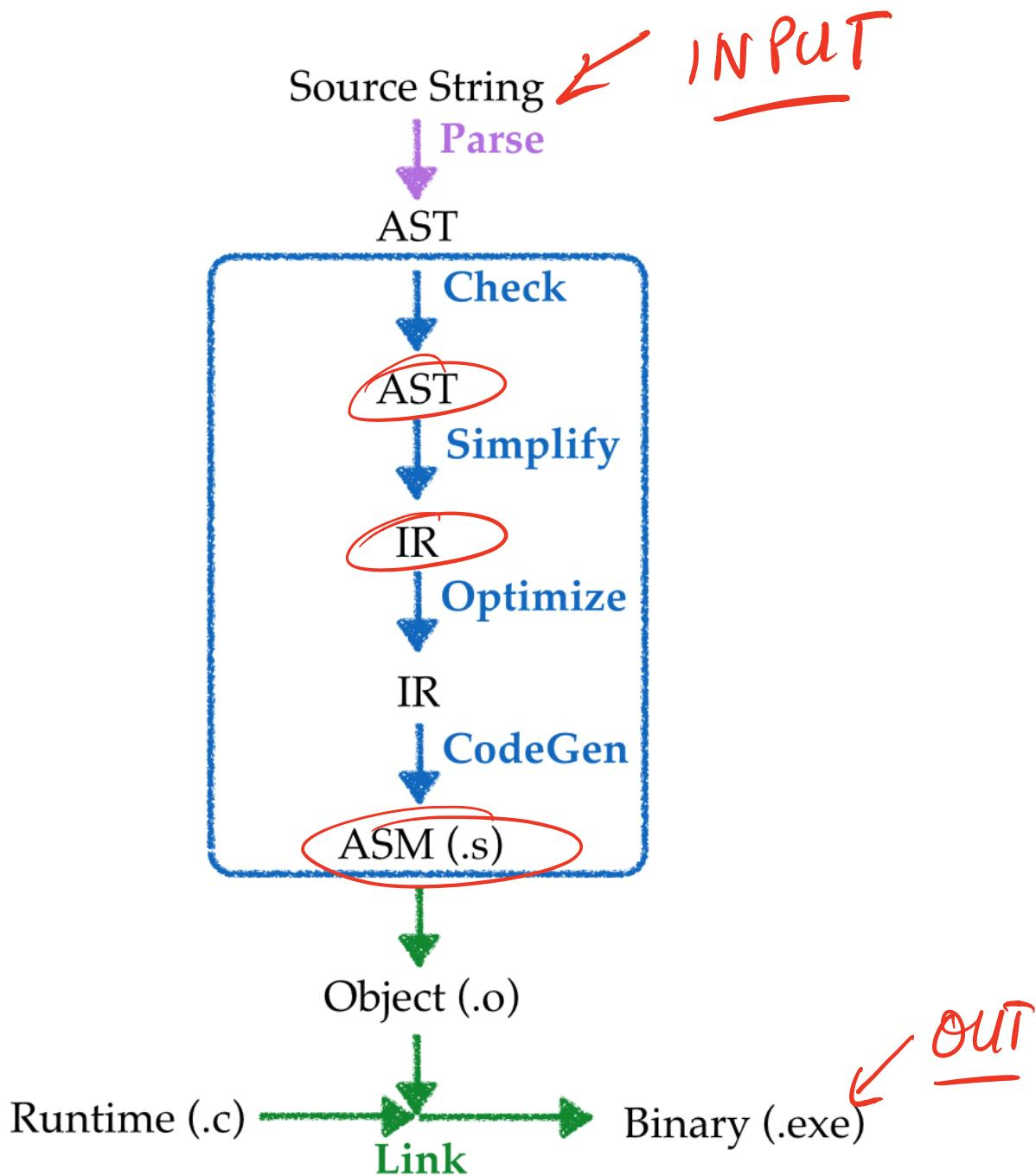
An input source program is converted to an executable binary in many stages:
